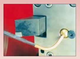
**LolliPop** nozzle shown installed in lathe turret.
